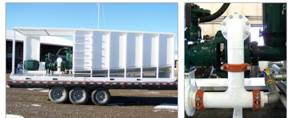
The finished product, dubbed the "shark tank", was built to separate and suspend fine particulate toward the top of the tank while drawing the clean, filtered water from the bottom.
